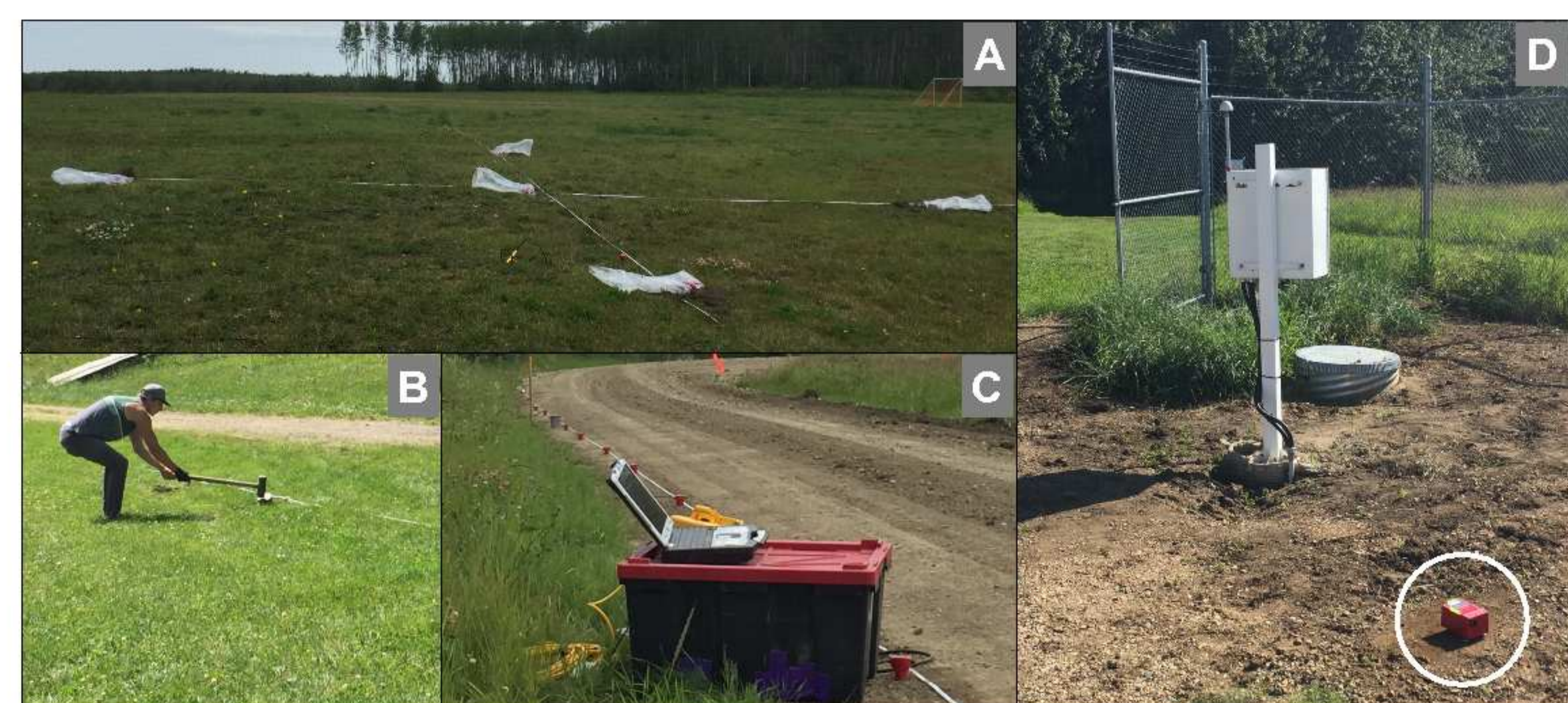
Figure 2 — Images from the summer 2016 field campaign. (A) A 5-sensor array deployed for ambient noise (passive) data collection at station RDEA. (B) and (C) demonstrate the implementation of the multi-channel analysis of surface waves (MASW) acquisition technique (active, impact source), and (D) a Tromino® (portable three-component seismograph) is used to record ambient vibrations and demonstrates the single-station MHVSR method implemented at station ATHA.
