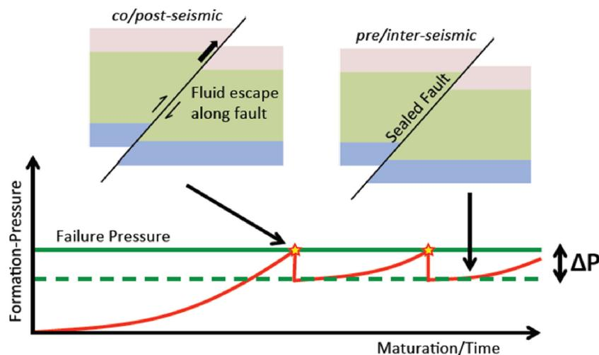
**Figure 4.** Model for the fault-valve cycle. Formation pressure builds up due to hydrocarbon generation and then is expelled due to co-seismic permeability enhancement.  $\Delta P$  denotes co-seismic pressure drop, here assumed to be constant for simplicity. Fault seal is gradually restored during interseismic intervals, thus re-initializing the cycle. Modified from MacKay (2015).
